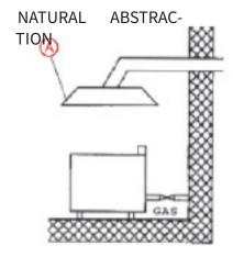
The hood is vented to a separate of the chimney body. The flue gas extraction is ensured by natural draft chimney
