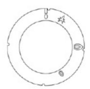
Turn the throttle knob to the \star position and keep it depressed. At the same time press the button 7 piezzo el. the flame will ignite automatically.
