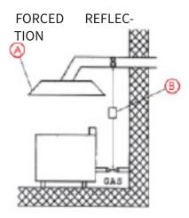
The hood is vented without natural exhaust. Exhaust fumes are extracted by means of a fan (forced exhaust). In this case it is necessary to provide a connection to the gas supply to shut off the gas supply in the event of a failure of the ventilation unit.
